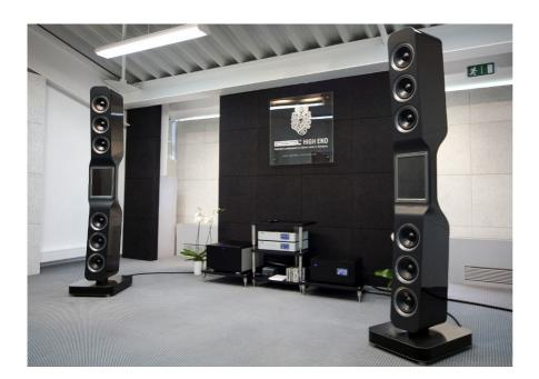
What the pictures don't reveal is that it's is a full dipole with not only front and rear output from the panel but three 7 inch bass drivers on both sides. The Epoque Fine is a 220lb speaker but Göbel was demonstrating the Epoque Reference which has the another six driver bass section above the panel and almost doubles that weight. Yet it's a system which sounded remarkably open, natural and even dynamic with a string quartet piece.
